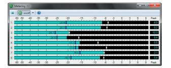
The CEDAR Cambridge Metering module is designed with reference to AES17, BS6840: Part 18: 1996 and IEC-60268-18.
